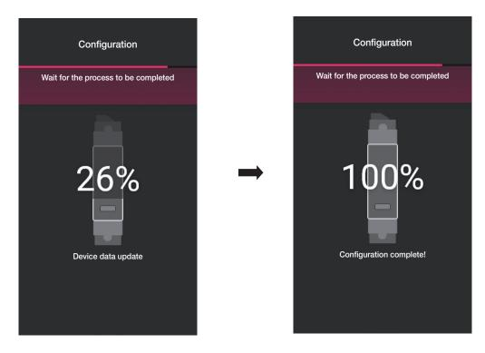
Meter configuration is now complete. The device association screen will now display the associated meter with the respective name and relevant environment.
