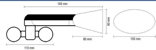
EN - Remove the two side covers. Place the base on the wall and mark the points to be drilled with a pencil. Drill and fix the plugs supplied, screw the base to the wall. Connect the sensor to the control panel.
